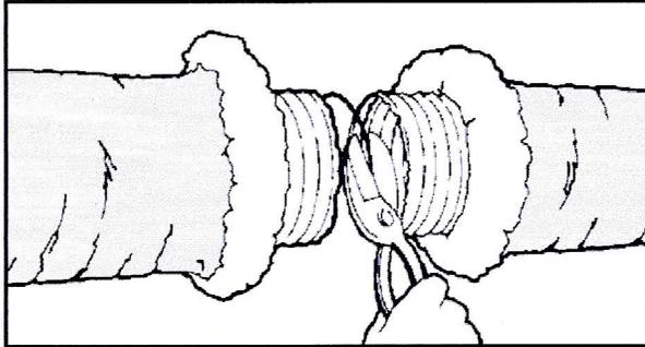
2. Slide at least 1" [25 mm] of core over fitting and past the bead. Seal core to collar with at least 2 wraps of duct tape. Secure connection with clamp placed over the core and tape and past the bead.
