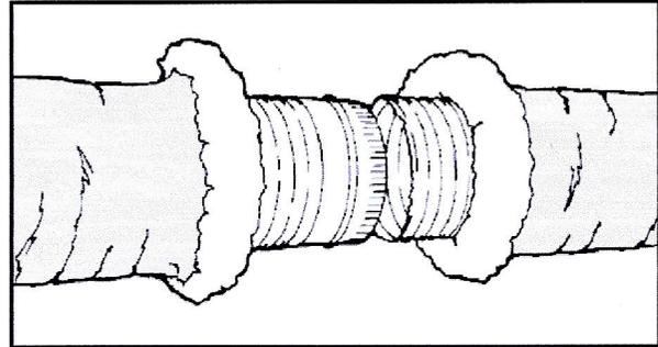
2. Tape cores together with at least 2 wraps of duct tape. Secure connection with 2 clamps placed over the taped core ends and past the beads.
